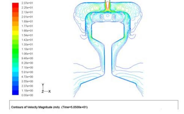
FIGURE 4 Streamlines pattern of Z=0 section
