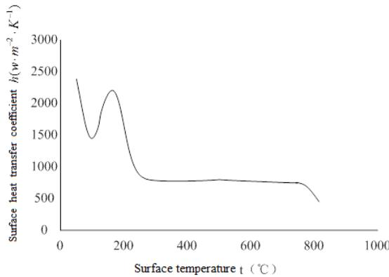
FIGURE 2 Surface heat transfer coefficient of air-cooling
