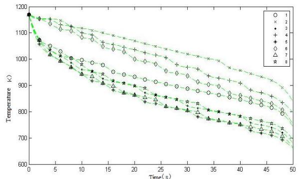
FIGURE 17 Temperature curve of hardened layer as time
