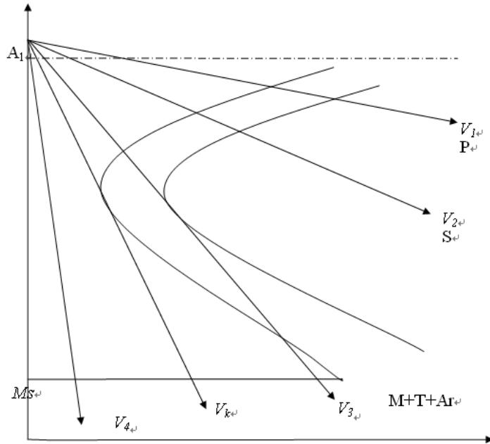
FIGURE 16 Austenite Isothermal Transformation Curve (C curve)
